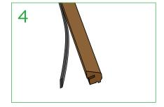
Apply strip of self-adhesive dry glaze tape to back edge of QW-GB5A (SD1A) bead. The tape should be at least 2 mm thick to ensure adequate compressive bond.
