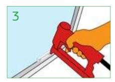
The clips can be fixed using staples, screws or pins. We recommend to use 2 x 80 series staples 12 mm (or longer if preferred) per clip. With the air gun regulators set at approx. 4 bar. Ensure fixings do not protrude into the clip channel and foul bead fitments.
