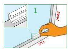
Fit glass panel safely into the frame as required. Offer clip QW-GCA to frame against glass ensuring the correct orientation.
