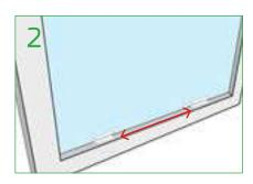
Ideal clip length is 50 mm and 75 mm (but longer length can be used if required). We recommend clips should be spaced at 150 mm intervals. This is a customer preference - the more clips the stronger the fixing.
