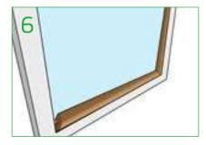
Repeat the process for the jambs and top. The beads will sit automatically in line with frame and should not protrude when pushed correctly onto the clips.
