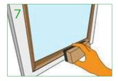
Using a felt covered block or a roller, gently apply pressure along each bead to ensure that they are firm in place and a good bond between the dry glaze tape and glass has been achieved.
