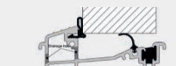
Stormguard AM370 Open In - NOT Part M Compliant 85, 150 or 180mm Special Reinforced Cills available
