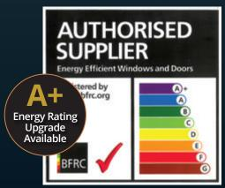
Energy Ratings - Calculation based on 'U' Value, air leakage and solar gain
