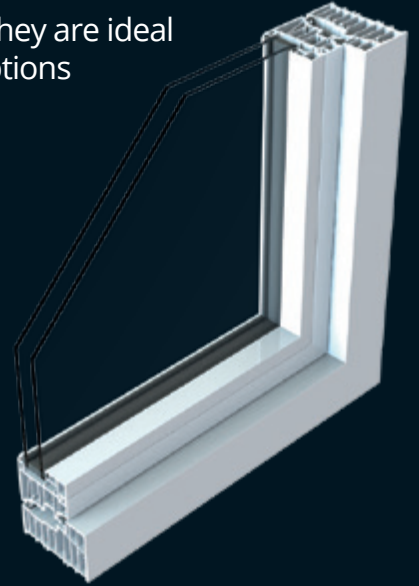
100mm 9 chambered energy efficient profile achieving 0.79 W/m²k U-Value for 28mm double glazing or 44mm triple glazing
